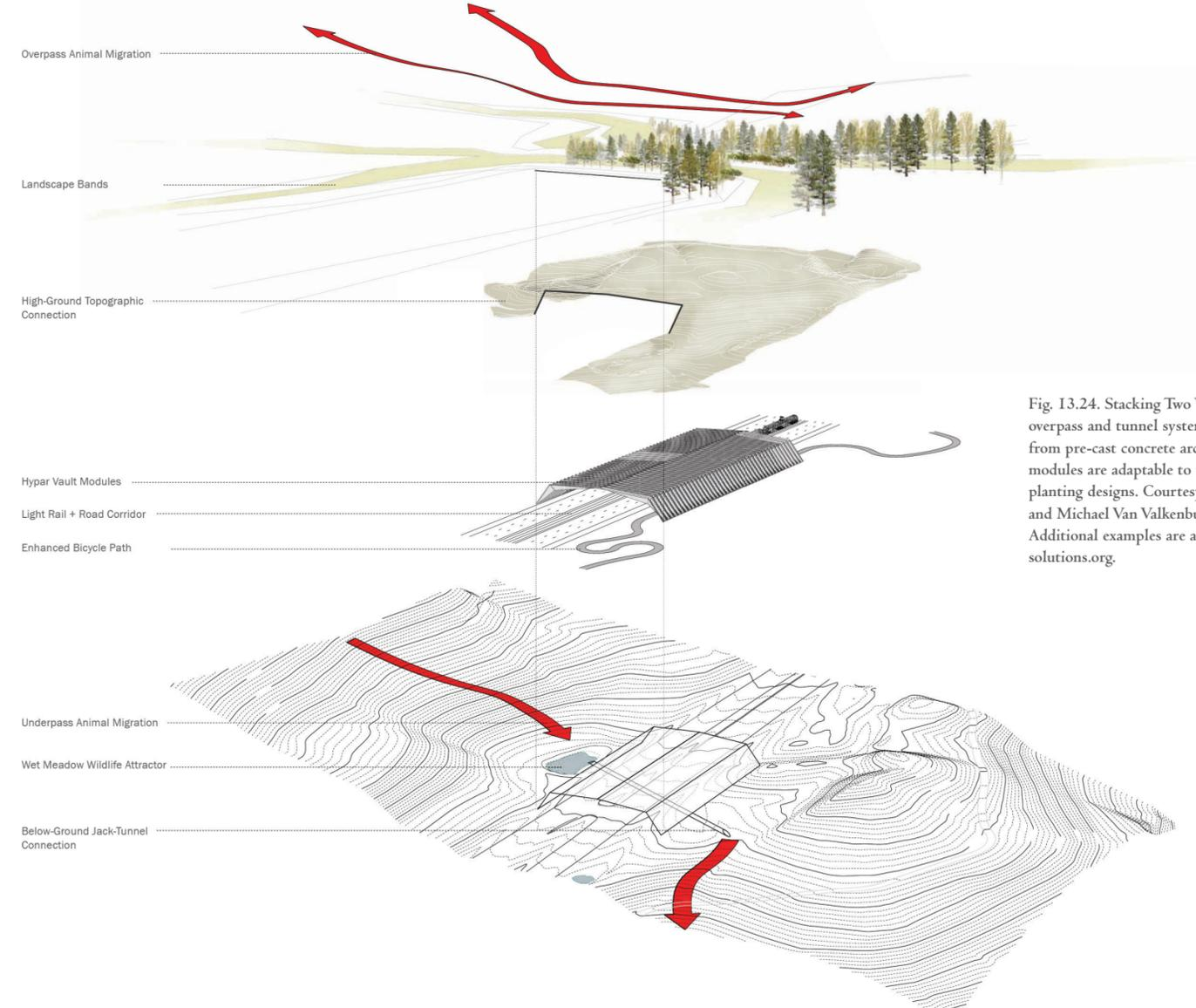
Fig. 13.24. Stacking Two Worlds: Here, an integrated overpass and tunnel system for large mammals is made from pre-cast concrete arches. The hinged, hypar-vault modules are adaptable to various site conditions and planting designs. Courtesy of HNTB Corporation and Michael Van Valkenburgh and Associates, 2010. Additional examples are available at <http://www.arc-solutions.org>.
